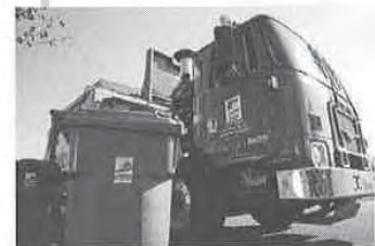
A hydraulic hybrid garbage collection truck consumes 33% less fuel than a traditional garbage truck
